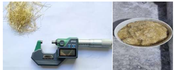
Steel Fibers : length=13 mm, Dia =0.15mm
